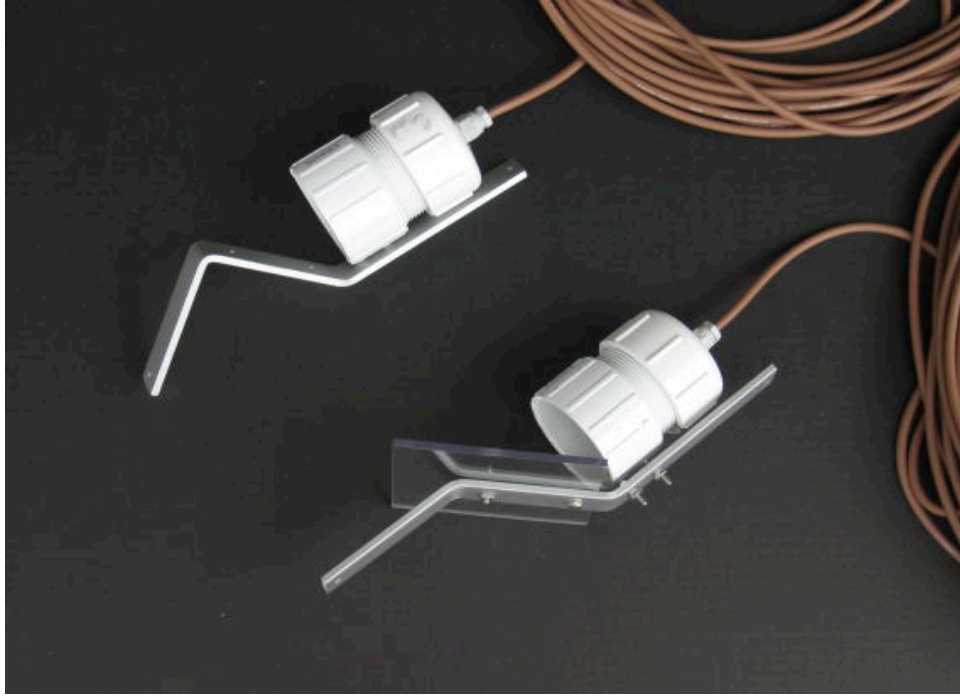
Figure 3. Examples of different bat-hat mounting systems used to deploy acoustic microphones at multiple heights on meteorological towers.
