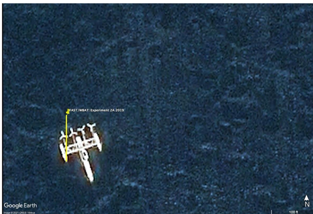
Figure 3.2.2: Deployment location of the WBAT echosounder mounted on the FAST platform, shown for Study 2A relative to the PLAT-I on a flooding tide. Length of yellow line represents the horizontal length from the optical camera deployed at the leading edge of the starboard pontoon to the position of the FAST platform: ~30 m.
