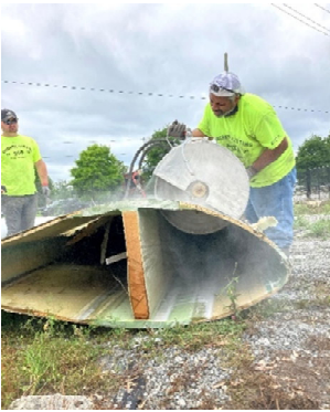
Figure 9: Large sections are cut into smaller test specimen
