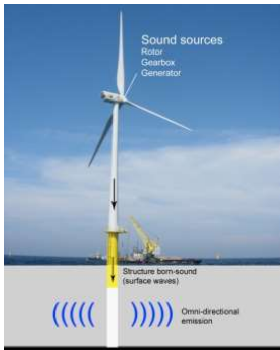
Figure 3 Basic sound propagation noise model of the structure-borne propagation path of rotational devices, gearbox, turbine and auxiliary engines.
