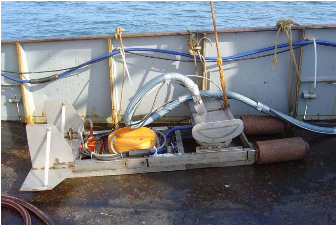
Photo 1. The towed body with the 200 kHz (left, orange) and the 38 kHz (right, yellow) transducers.
