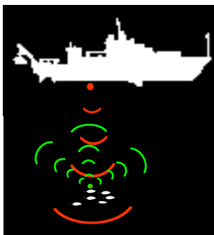
Figure 2.3. Method of echo location. An acoustic signal is sent by the transducer and will reflect on structures in the water such as fish, plankton and the bottom.
