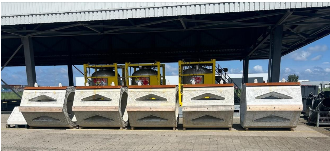
Figure 4. The five ExoLodges and the ExoAnchor control block prior to deployment.
