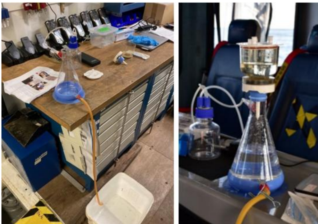
Figure 11. Water filtration kit used to filter eDNA from seawater samples.
