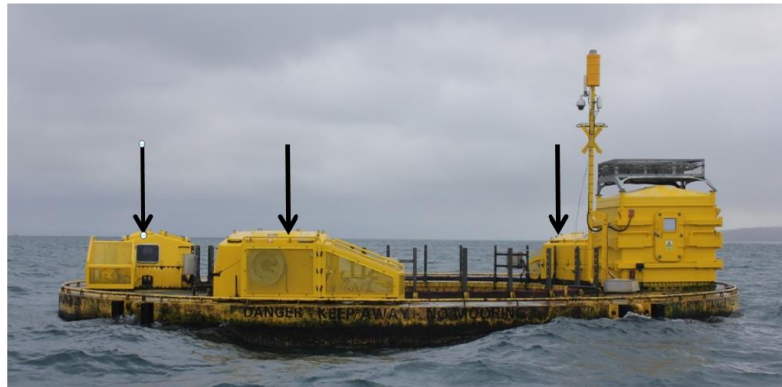
Fig.1: The Fred.Olsen BOLT Lifesaver wave energy converter deployed at FaBTest. The PTOs are marked with downward arrows. Picture credit: 2013 Duncan Paul, Falmouth Harbour Commissioners
