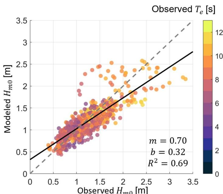
**Figure 6.** Modeled (y-axis) versus observed (x-axis) significant wave heights ( $H_{m0}$ ) for each measurement of the deployment period. Colors indicate the observed wave energy period ( $T_e$ ). Linear regression best fit for wave heights is given as a black line with slope ( $m$ ),  $y$ -intercept ( $b$ ), and goodness-of-fit ( $R^2$ ), provided in the bottom right. A 'perfect' 1:1 ratio is shown as a dashed gray line.
