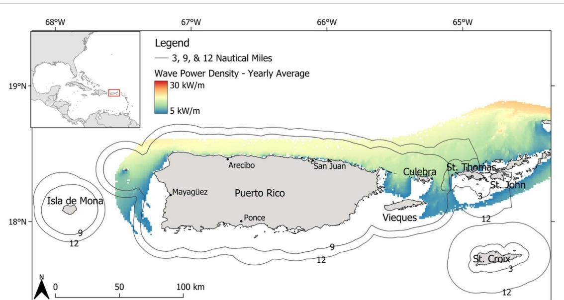
**Figure 1.** Annual wave power density around Puerto Rico and the US Virgin Islands between  $5 \text{ kW m}^{-1}$  (blue) and  $30 \text{ kW m}^{-1}$  (red). Dark grey lines represent the 3 nm (US Virgin Islands) and 9 nm (Puerto Rico) state and 12 nm federal water boundaries.
