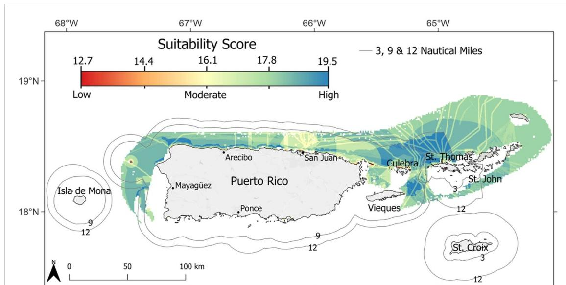
**Figure 3.** Heatmap of suitable areas to co-locate wave energy and offshore integrated multi-trophic aquaculture. The map is clipped to display only areas with suitable wave power density ( $5\text{--}30\text{ kW m}^{-1}$ ).
