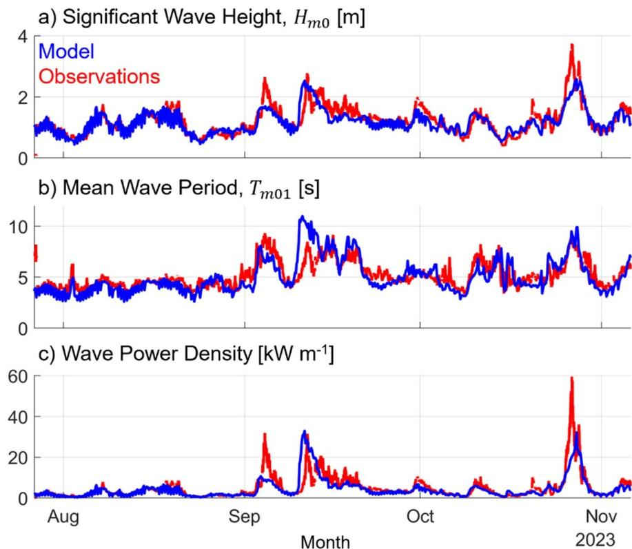
**Figure 5.** Model (blue) versus observed (red) significant wave height,  $H_{m0}$  (a), mean wave period,  $T_{m01}$  (b), and wave power density (c), over the duration of the Sofar Spotter buoy deployment (x-axis).
