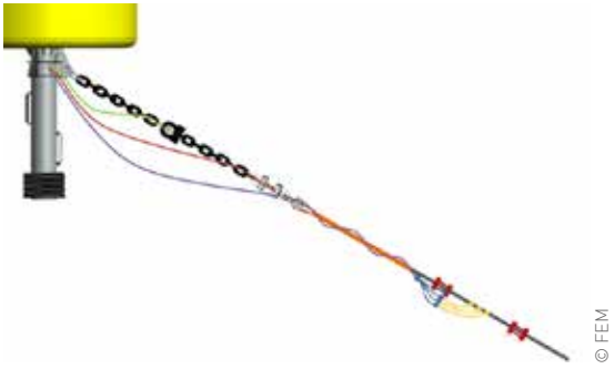
| Detailed view of the mooring of the MONABIOP demonstrator
