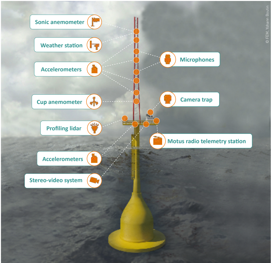
Instrumentation already in place on the met mast
