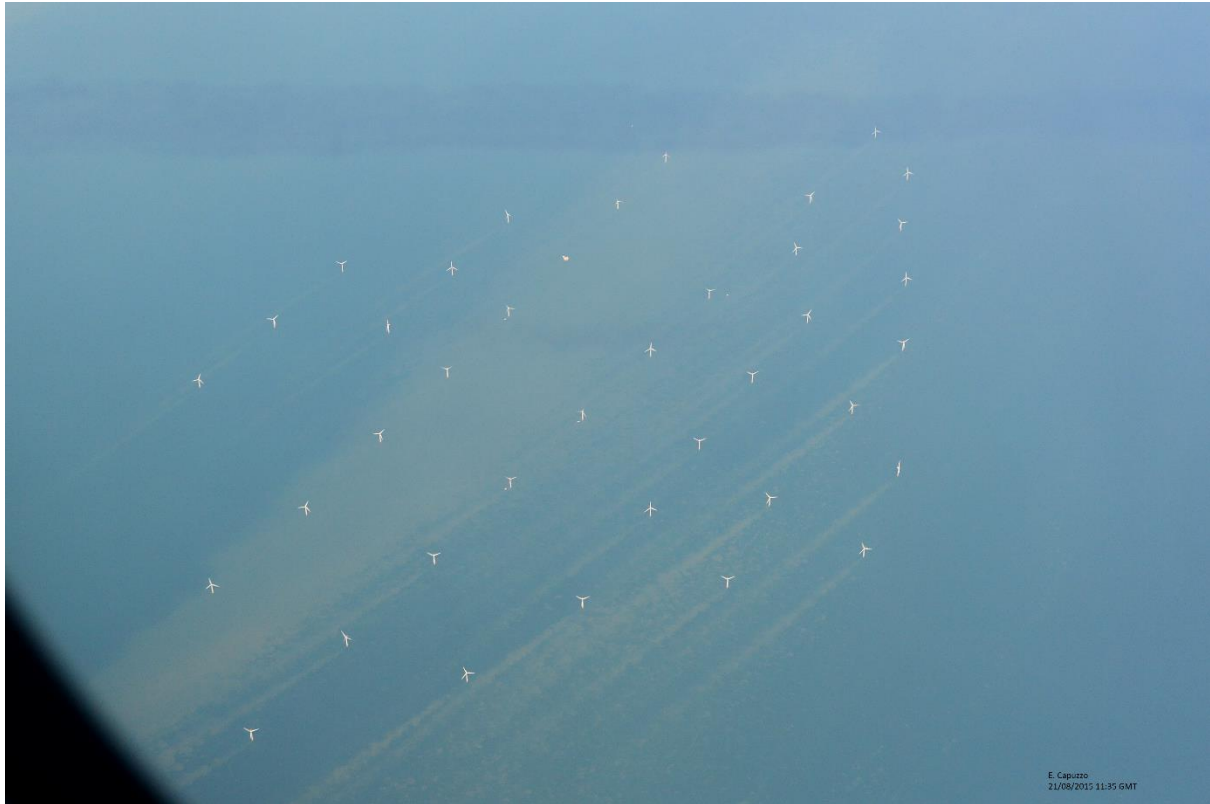
Figure 1 Wake formation associated with individual monopiles of the Greater Gabbard wind farm
