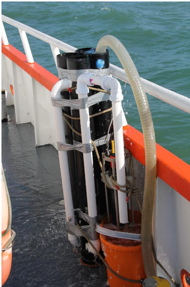
Figure 19 Deck sampling rig for continuous measurement of suspended sediment load, temperature and salinity.
