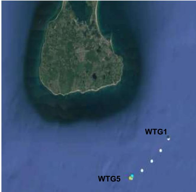
**Figure 10: Image of Block Island wind turbine area. The wind turbine generators are indicated in white, the horizontal line array placement in cyan at WTG5, and the vertical line array in gray at WTG1.**
