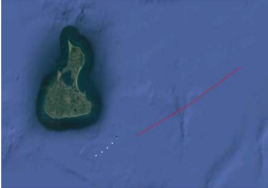
**Figure 18:** This figure shows the Block Island area. The five turbines are marked in white, and the vertical line array is marked in gray at turbine #1. The red line is the track of the R/V Tioga towing a sound source for playback operations.
