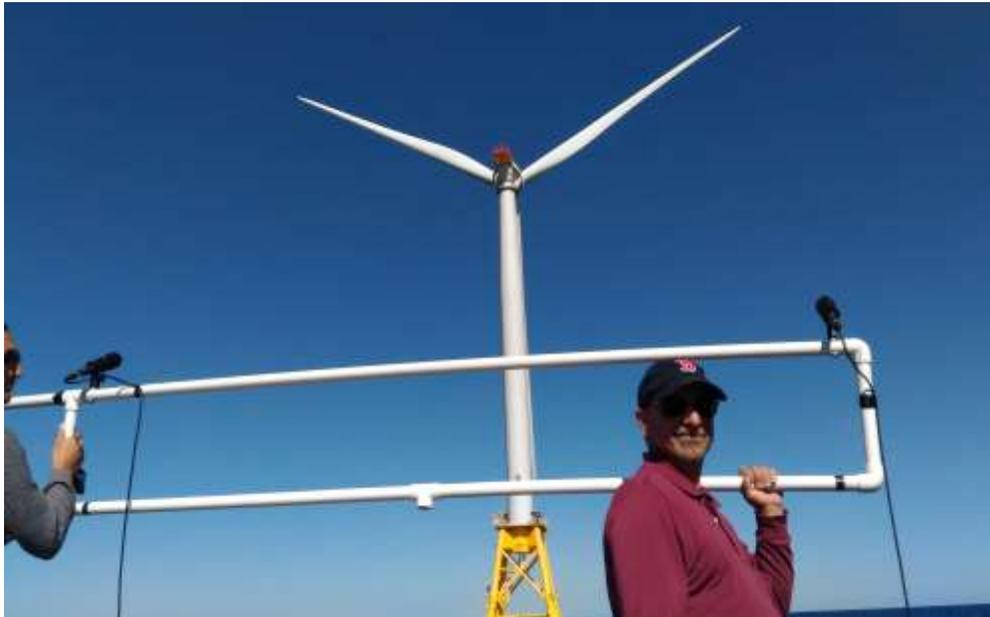
**Figure 24: Holding the omni-directional microphone array at WTG1.**
