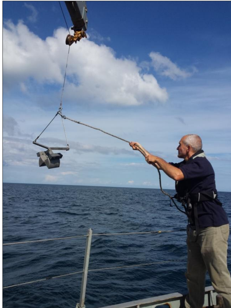
Figure 3.5 –Van Veen sediment grab deployment from 'Boy Brendan'
