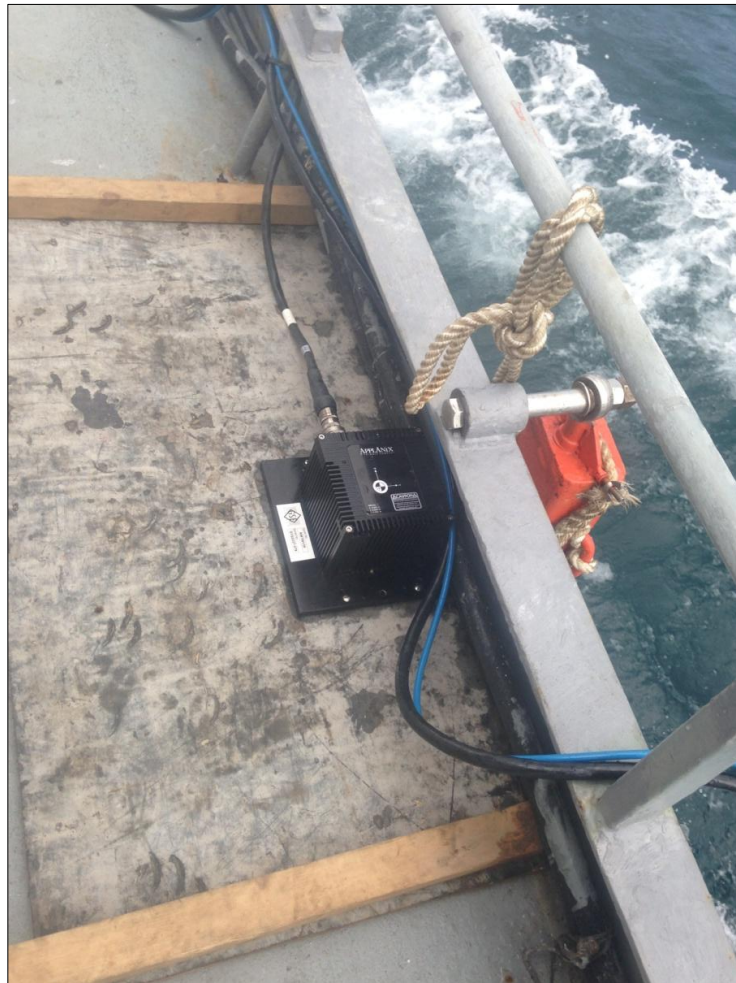
Figure 2.3 – POS MV IMU shown in secure mounting position on starboard side ('Boy Brendan')
