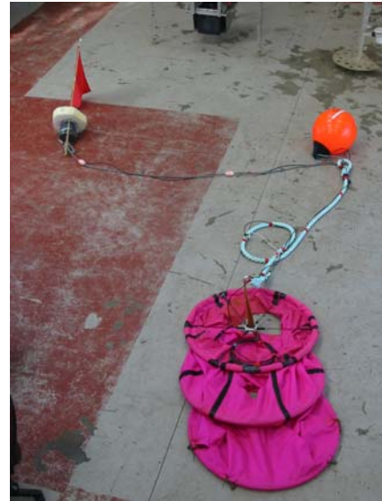
Figure 6 Drifting acoustic drogue set up. (Note: drogue-to-float line is looped over to fit drogue in photograph).
