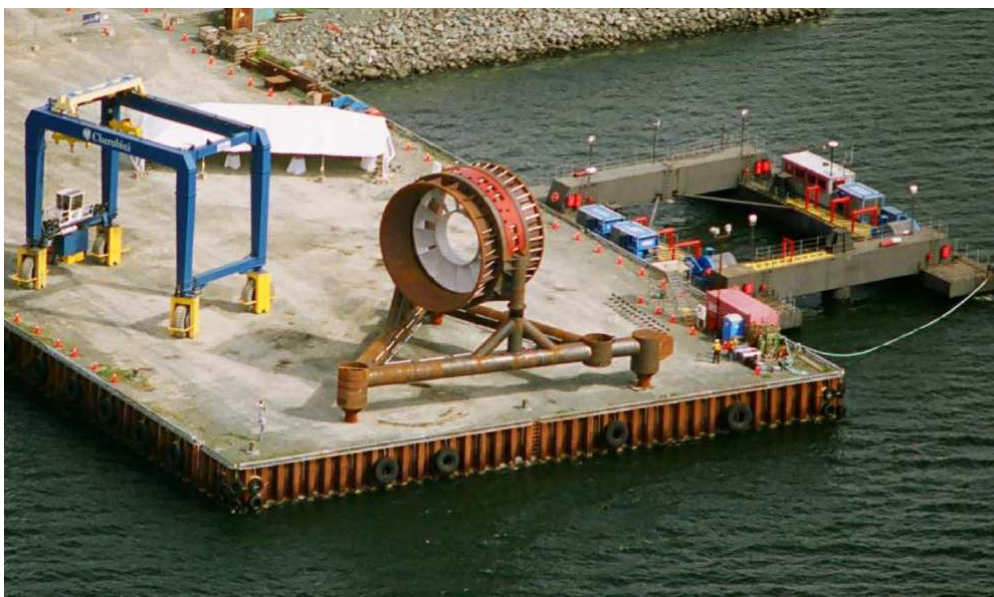
Figure 50 OpenHydro turbine prior to installation in Bay of Fundy [55]
