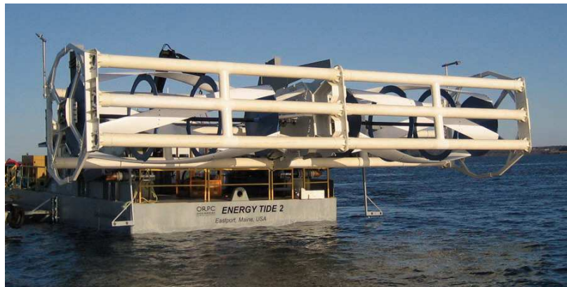
Figure 70 Beta Pre-Commercial TidGen Power System during testing at Cobscook Bay [97]
