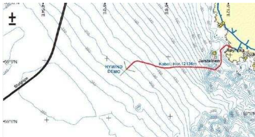
Figure 17 Sub-sea cable route at METCentre [24]
