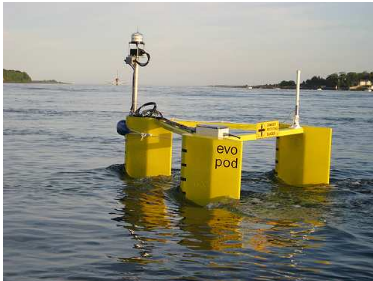
Figure 57 Evopod installed in Strangford narrows with SeaGen tidal turbine visible in background[74].
