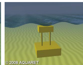
© 2008 AQUARET Point Absorber (left) and Submerged Pressure Differential Device: prime mover is floater against reference body
