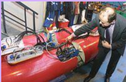
Hydraulic PTO of the Pelamis 1:7 scale model (Photo: Pelamis Wave Power Ltd)
