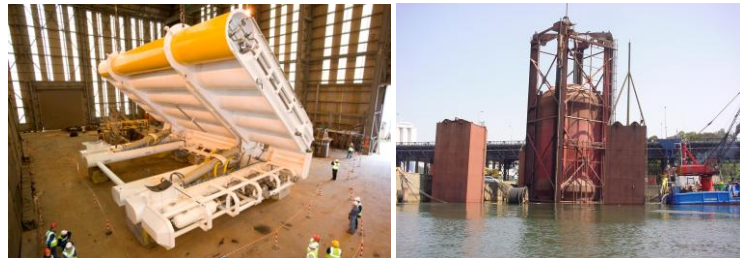
Oyster – Dry Test of the PTO (Left photo: Aquamarine Power) and AWS – Test of Auxiliary Systems and instrumentation at the Harbour (Right photo: Teamwork Technology B.V.)
