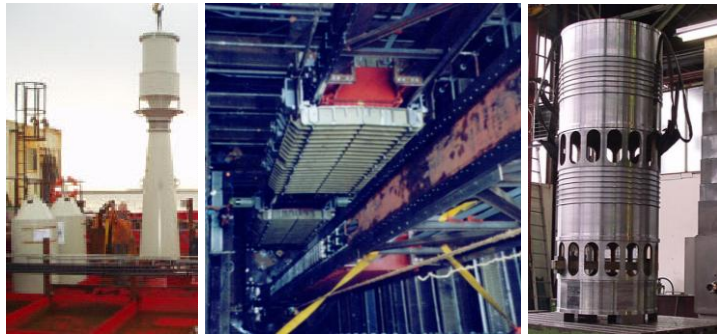
Wave Dragon 2.6kW Low Head Turbines (left photo: Wave Dragon ApS), AWS 2MW Linear PM Generator (mid photo: Teamwork Tech. B.V.) and AWS Water Brake Valve (right photo: Teamwork Tech. B.V.)
