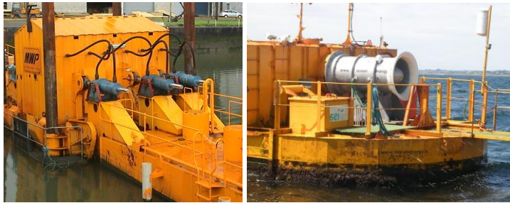
McCabe Wave Pump Hydraulic Rams (left photo: Hydram Tech. Ltd) and OE buoy 15kW Wells Turbine (right photo: OceanEnergy Ltd)
