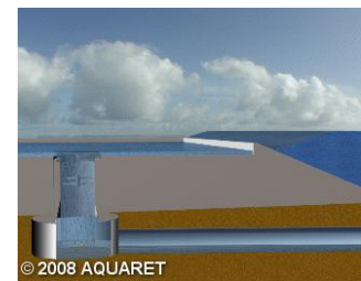
© 2008 AQUARET Overtopping: prime mover is combination of barge/ramp and basin surface
