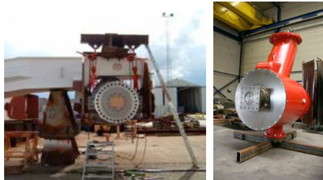
Seagen 600kW Induction Generator (left photo: Marine Current Turbine Ltd) and Tocado 30kW PM Generator (right photo: Tocado Inter. B.V.)
