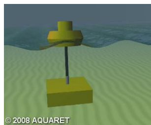
© 2008 AQUARET Point Absorber (left) and Submerged Pressure Differential Device: prime mover is floater against reference body
