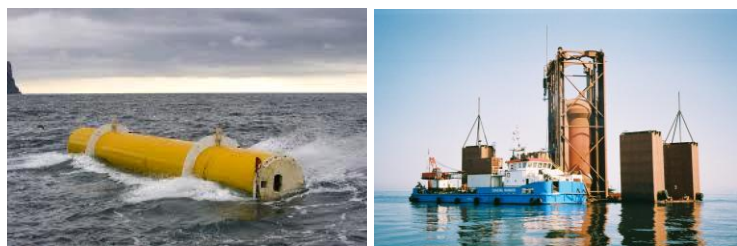
Full Scale (315kW) Oyster prototype in operation at Orkney, Scotland (Left photo: Aquamarine Power) and Full Scale (2MW) AWS prototype during deployment offshore at North Portugal (Right photo: Teamwork Technology B.V.)
