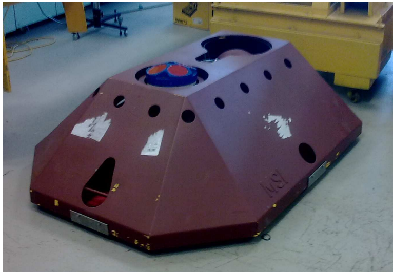
Figure 2: Example of an anti-trawl ADP bottom-mounting.
