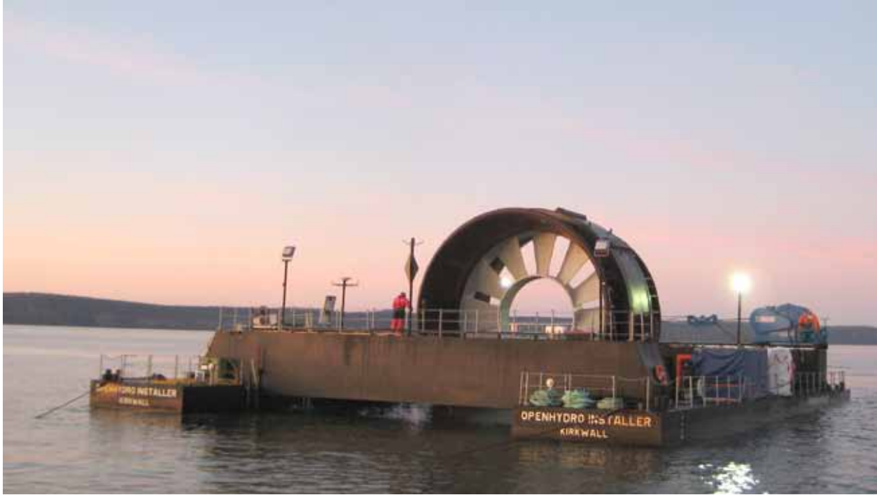
Figure 8 – OpenHydro 10 m (1 MW peak power) Bay of Fund Turbine (Source: OpenHydro)
