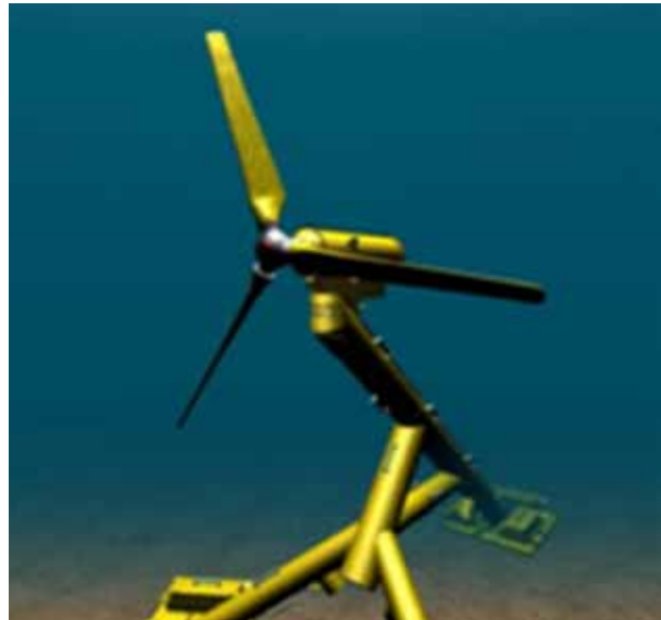
Figure 4 – Tidal Stream Turbine, Hammerfest Strom UK (Source: EERE 2010)
