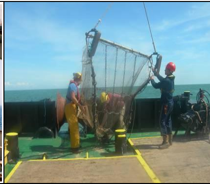
Plate 2: 2 m beam trawl
