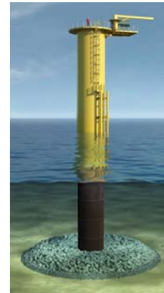
Figure 4-5: Typical monopile foundation (Courtesy: Ramboll)
