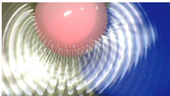
Figure 8. Scattering, radiation and strong interaction of a vibrating HSD, Elmer et.al. (2011).
