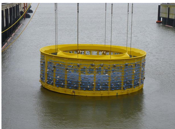
Fig. 18. HSD-box hanging on 8 ropes.
