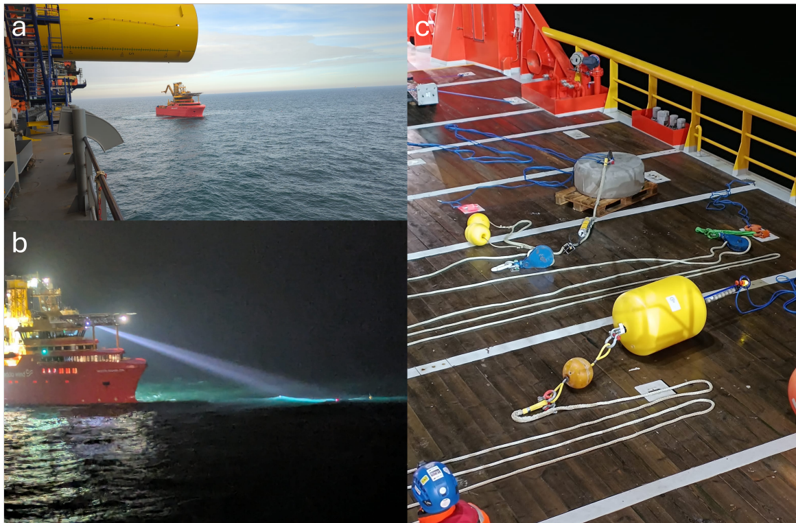
Figure 1.2: Impression measurement campaign works from the Vestri Enabler. a) The SOV in the field close by the Boreas during deployment of the setup. b) Setup retrieval at night. c) Setup laid out on deck. The snatch blocks were used for deployment.
