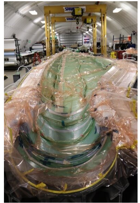
Figure 15. Construction of a revolutionary 13-meter thermoplastic blade at NREL's Composites Manufacturing Education and Technology Facility. A vacuum bag covers the laminate and mold, which is infused with resin. This blade is specifically designed to be recycled at the end of its service. Photo by Ryan Beach, NREL 62034
