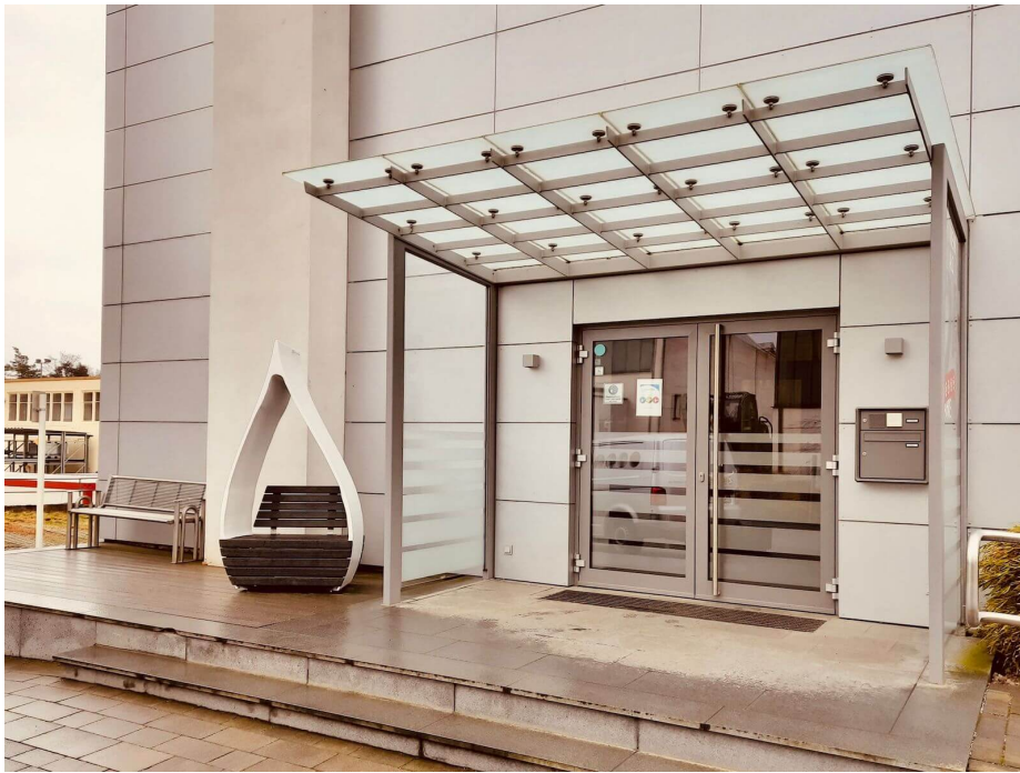
Figure 14. Wind turbine blades can be repurposed into a wide variety of applications. The example shows a repurposed blade that has been used to create outdoor seating. Photo from Anmet
