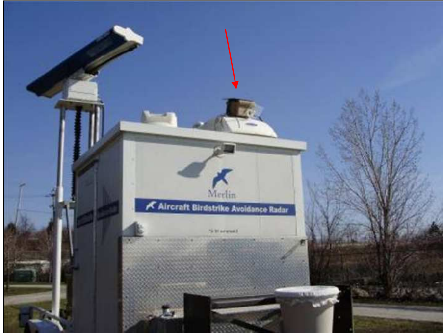
Figure D.7 Radar detector at onshore location, spring 2010
