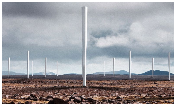
Figure 7: Vortex Bladeless Turbine (Ambrose, 2021)
