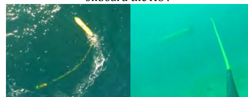
Fig. 5: AUV-towed magnetometer. (a) Aerial view, (b) View from the towed sensor
