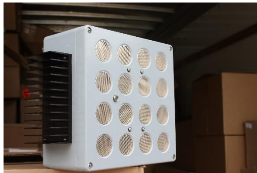
Figure 3. An ultrasonic deterrent device used in Arnett et al. 2013 (Photo by E. B. Arnett)
