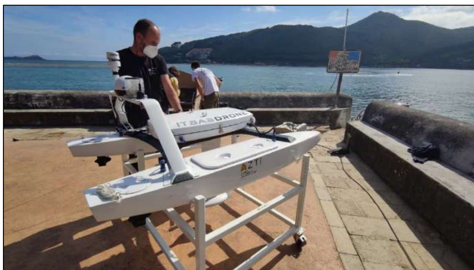
Figure 1. ITSASDRONE, an autonomous marine surface drone (Source: AZTI).
