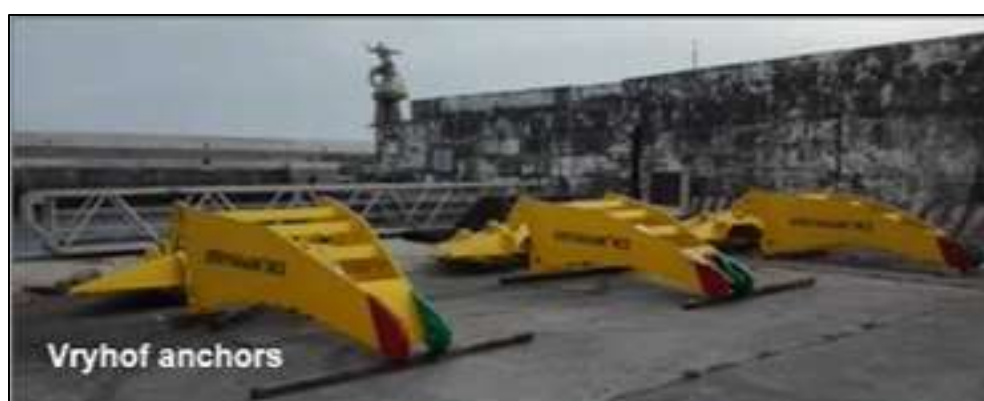
Figure 10. Drag Embedment Vryhof anchors utilized (Source: Tecnalia).
