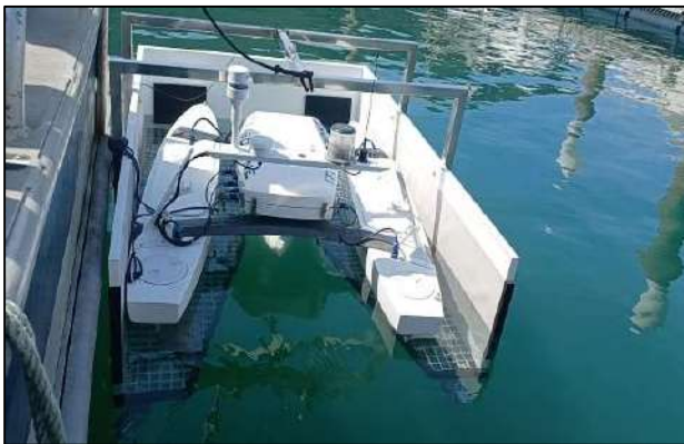
Figure 13. a) ITSASDRONE inside the docking station, b) ITSASDRONE towed by OLATU yacht (source: AZTI).
