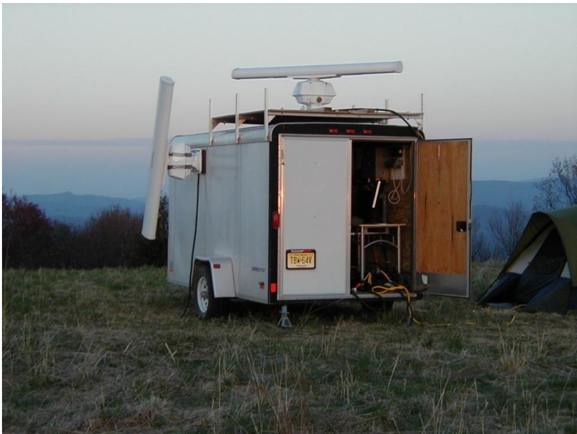
Figure 3. NJAS radar trailer, Highland Wildlife Management Area, Highland Co., VA. The tent houses a generator, which powers the radar and computers.
