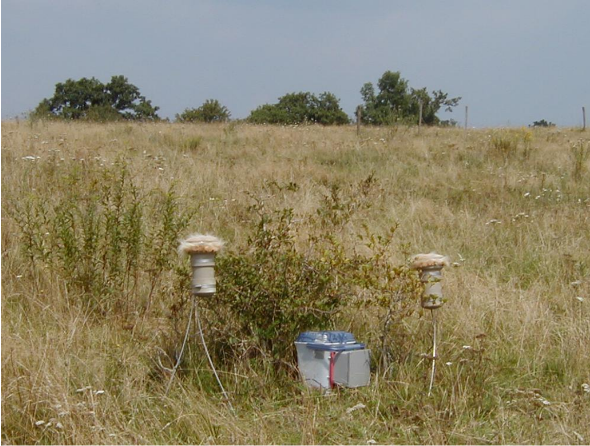
Figure 2. Autonomous recording unit (ARU), Allegheny Battlefield, Monongahela National Forest, Pocahontas County, WV. Microphones, two per unit, are nestled in PVC housings covered by shag wind screens. Sounds are recorded onto an mp3 recorder with 100 GB hard drive, housed in a weather-tight access box mounted on a bucket that holds the batteries. Each unit can record continuously for up to 65 days.
