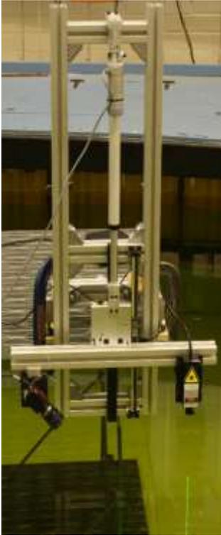
**Figure 30: Picture of the calibration rig used for the optical wave probe.**
