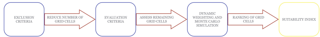
Figure 6. Flow chart of the suitability index methodology, showing exclusion screening followed by multi-criteria evaluation.
