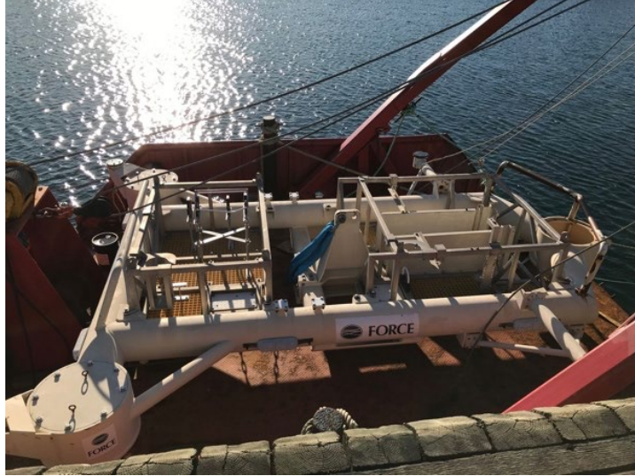
Figure 3: Calm water testing of the deployment and recovery procedure for FAST- 1 from Nov. 19, 2019, in Grand Passage.
