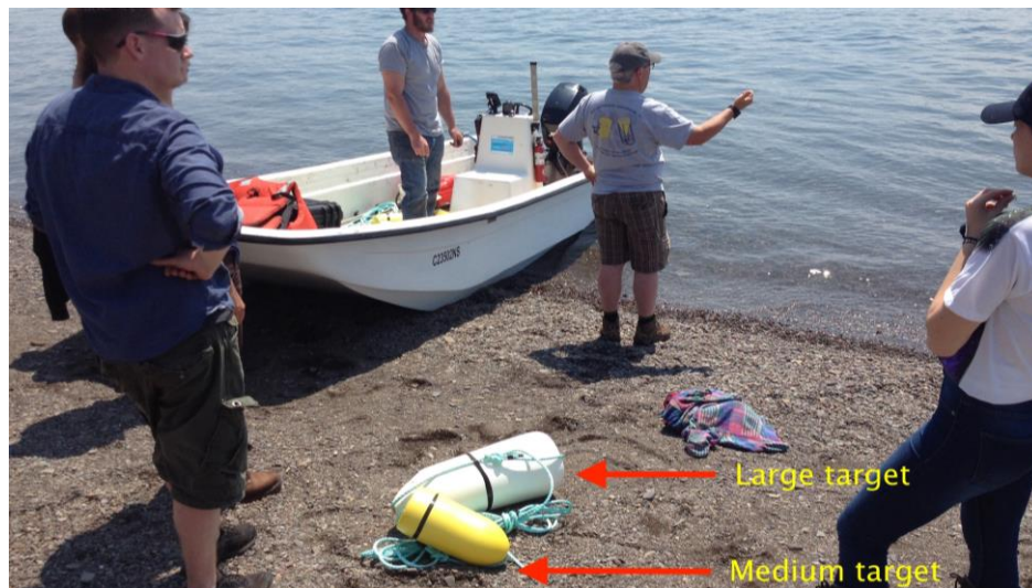
Figure 4: Preparing for low flow testing. The targets were deployed at different locations using the pictured vessel. As discussed in the main text, the large target was very well discerned up to 30 m range and across all bearings, even with Gemini noise present.
