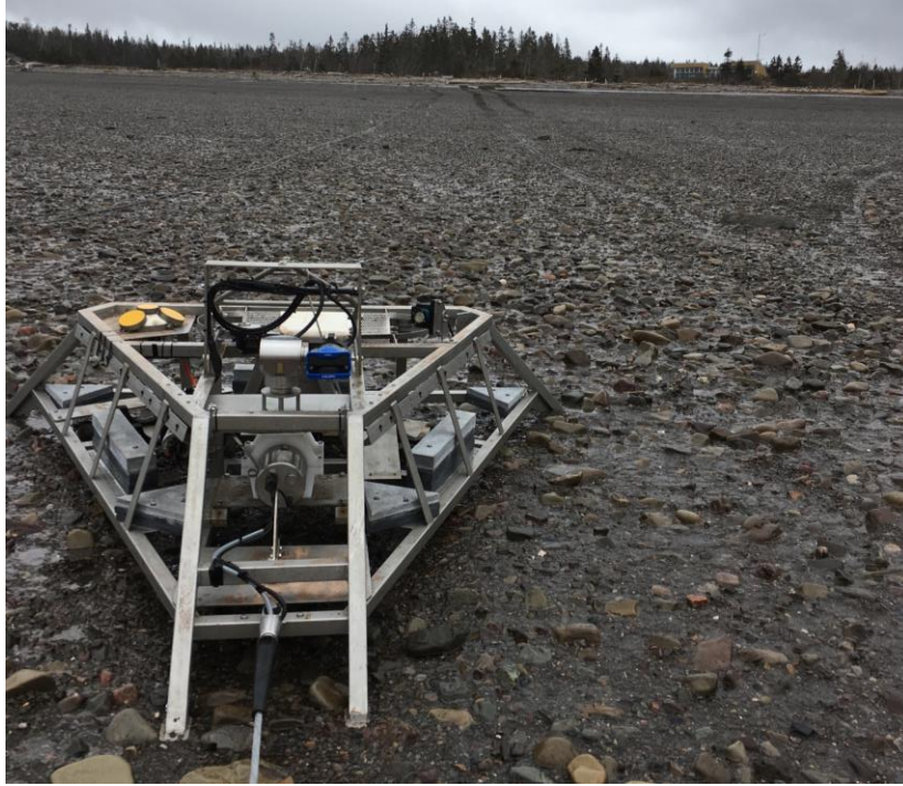
Figure 7: FAST-EMS in position for intermediate flow testing, far from the FORCE beach berm.
