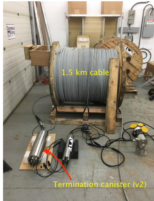
Figure 3: Electrical integration of FAST-EMS. Left: Testing of the sensor suite (Gemini not pictured). Right: Testing with the 1.5 km FO cable and new term can, which houses both power conditioning components and power and fibre connections between the FO cable and MUX.
