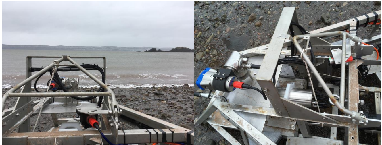
Figure 2: The results of mechanical integration of FAST-EMS, focused on maximizing the Gemini's range of view.
