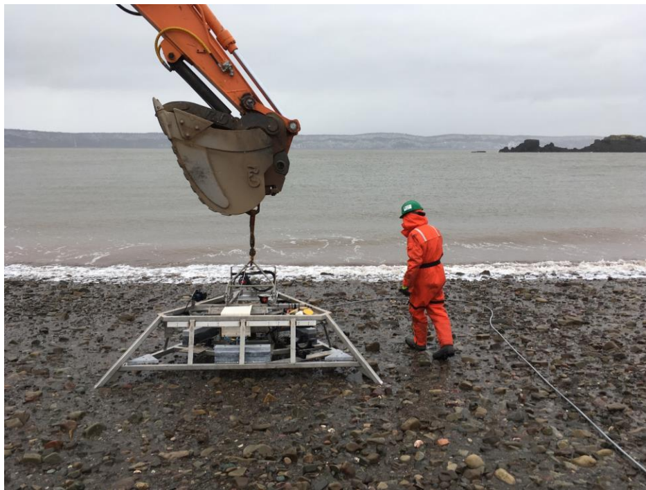
Figure 6: Deployment, by excavator, of FAST-EMS for the intermediate flow test.
