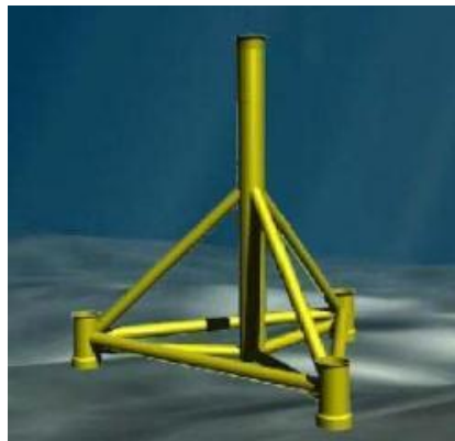
Drilled pin pile tripod
