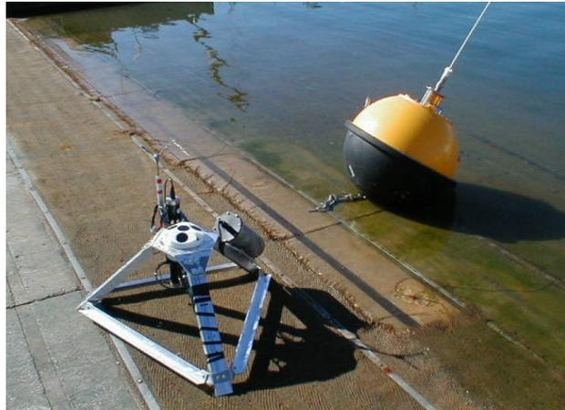
Figure 8. Nortek AWAC mounted in a bottom lander & a Datawell Waverider buoy (Pedersen and Lohrmann 2004)
