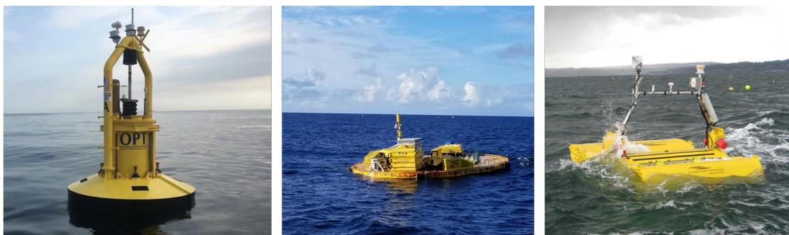
Figure 11. Point-absorber WECs currently deployed and/or in development, from left to right: Ocean Power Technologies’ PowerBuoy3, Fred Olson Lifesaver, and Columbia Power Technologies’ SeaRAY
