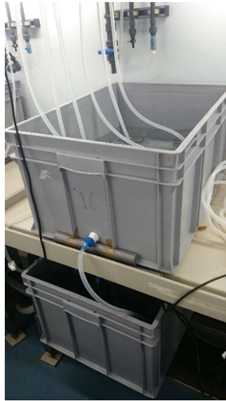
Figure 2.1. An experimental tank (top) and sump (bottom) for the crab physiology experiment.
