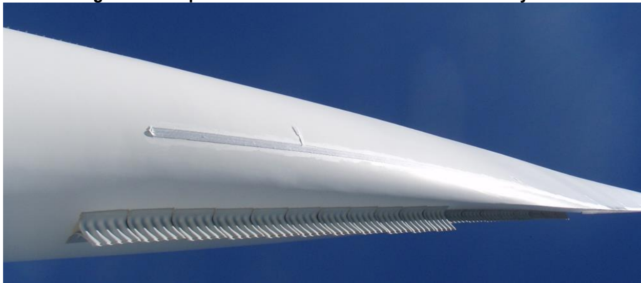
Figure 7: Completed Blade Installation of Strike-Free™ System
