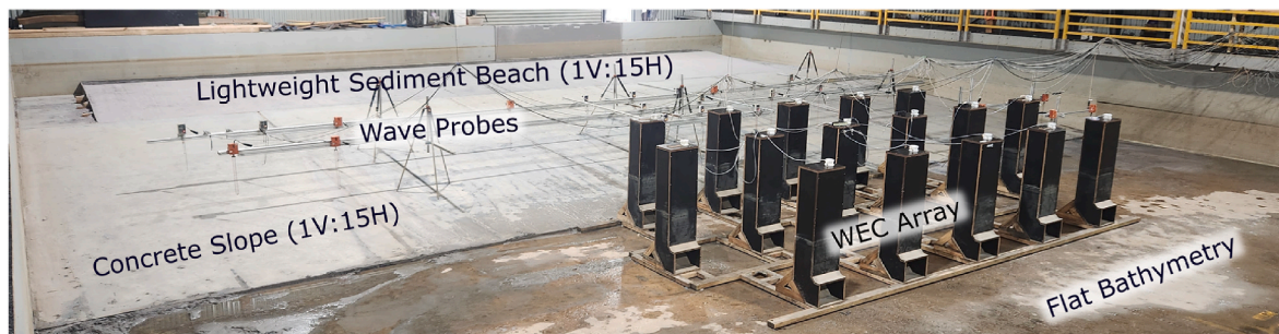
Fig. 2. Looking landward in the wave basin showing the three different bathymetry sections. The mobile sediment ‘beach’ section was reset to the same 1V:15H slope of the adjacent sloping concrete section prior the start of each test. The particular WEC array configuration shown here is ‘Regular: Three Row’ (refer to Section 2.3 and Fig. 7).
