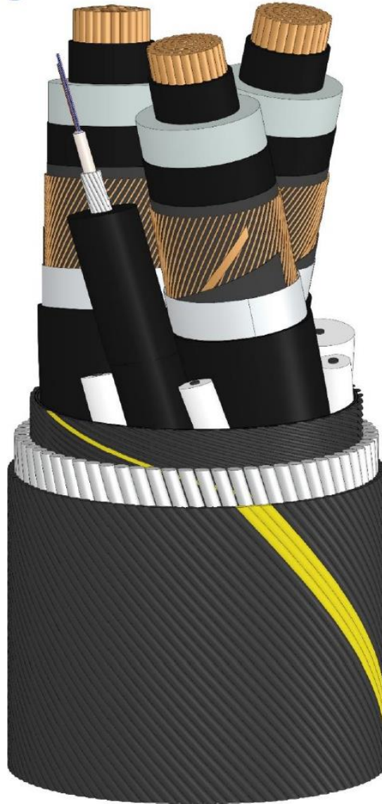
Figure 3.3-6. Representative Cross Section of an Inter-Array Cable
