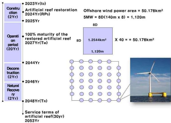
Fig. 3 Factors used in the HEA Analysis for Ulsan Floating Offshore Wind Power Complex
