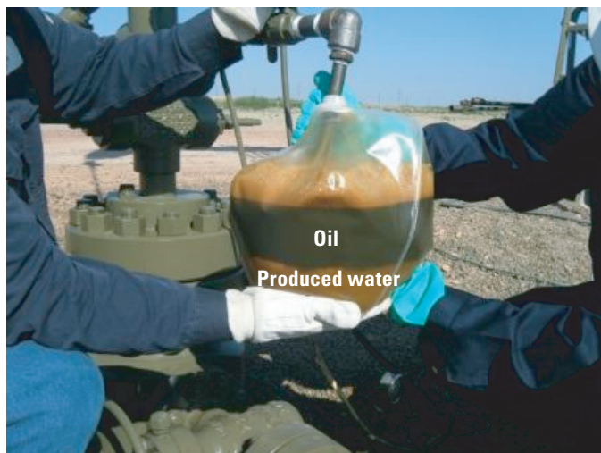
Figure 52. Oil and produced water collected from an unconventional Bakken Formation production well near Sidney, Montana, August 2014. Photograph by Gregory Delzer, U.S. Geological Survey.
