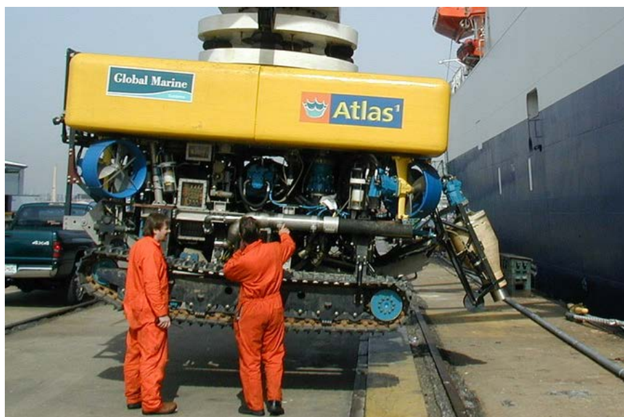
Figure 3.35 Example of an ROV equipped with a jetting system
