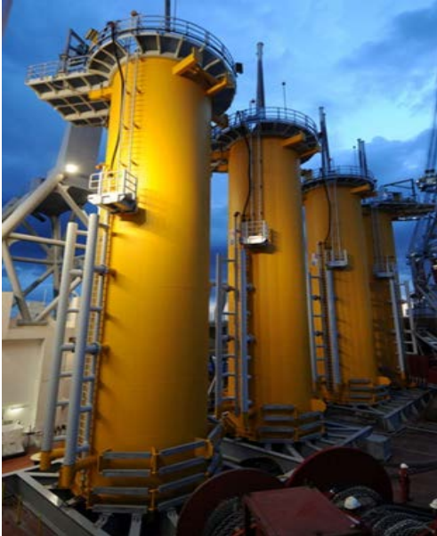
Figure 3.17 Typical wind turbine transition pieces
