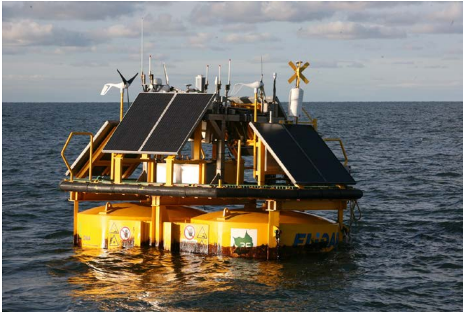
Figure 3.54 Example of a floating meteorological monitoring station, including wind lidar
