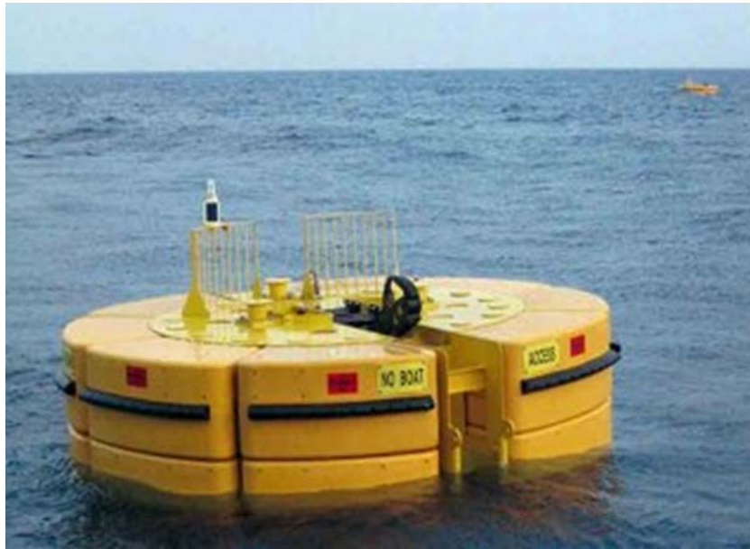
Figure 3.55 Illustrative example of a single buoy mooring
