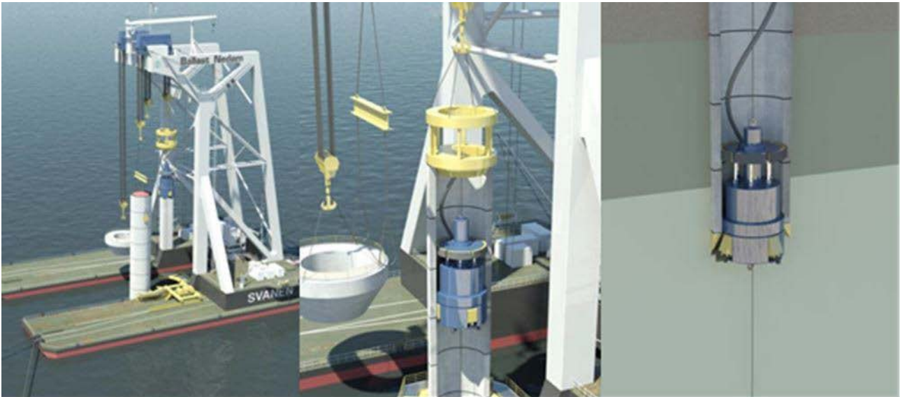
Figure 3.6 Illustrative visualisation of the installation of a concrete monopile foundation
