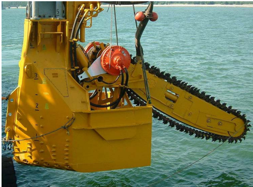
Rocksaw trencher, courtesy of Global Marine Systems
