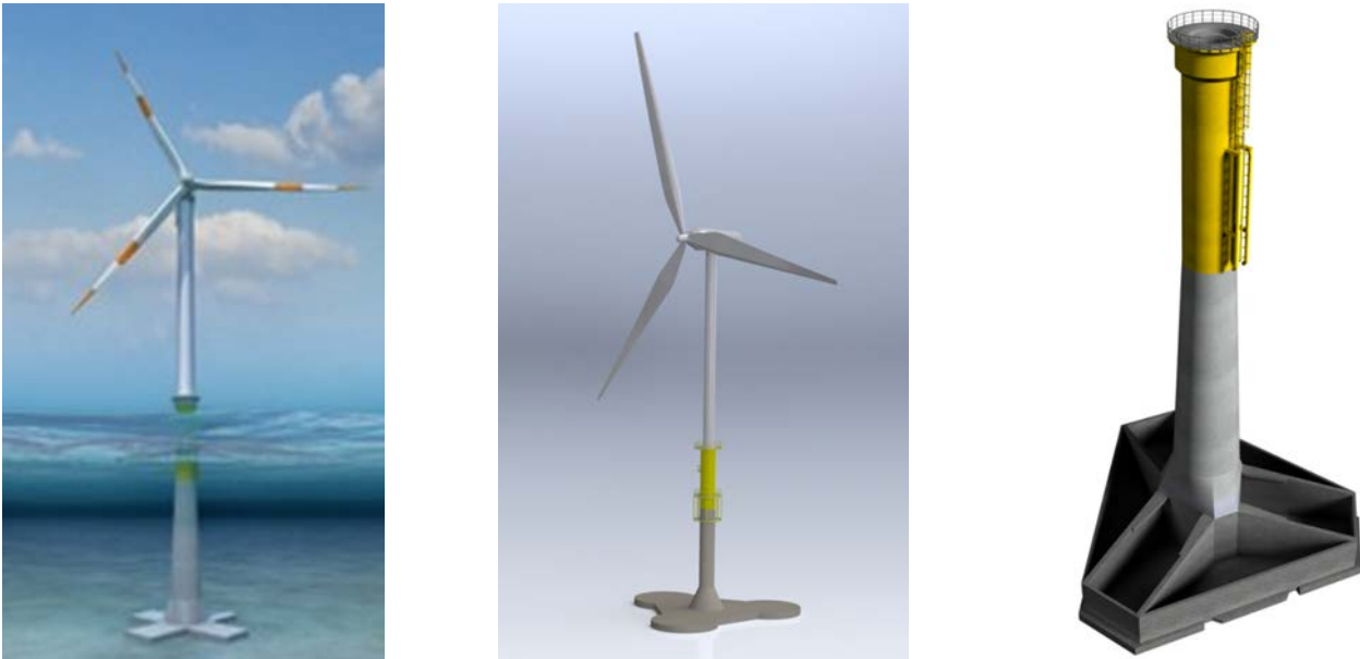
Figure 3.14 Illustrative examples of flat based gravity foundations
