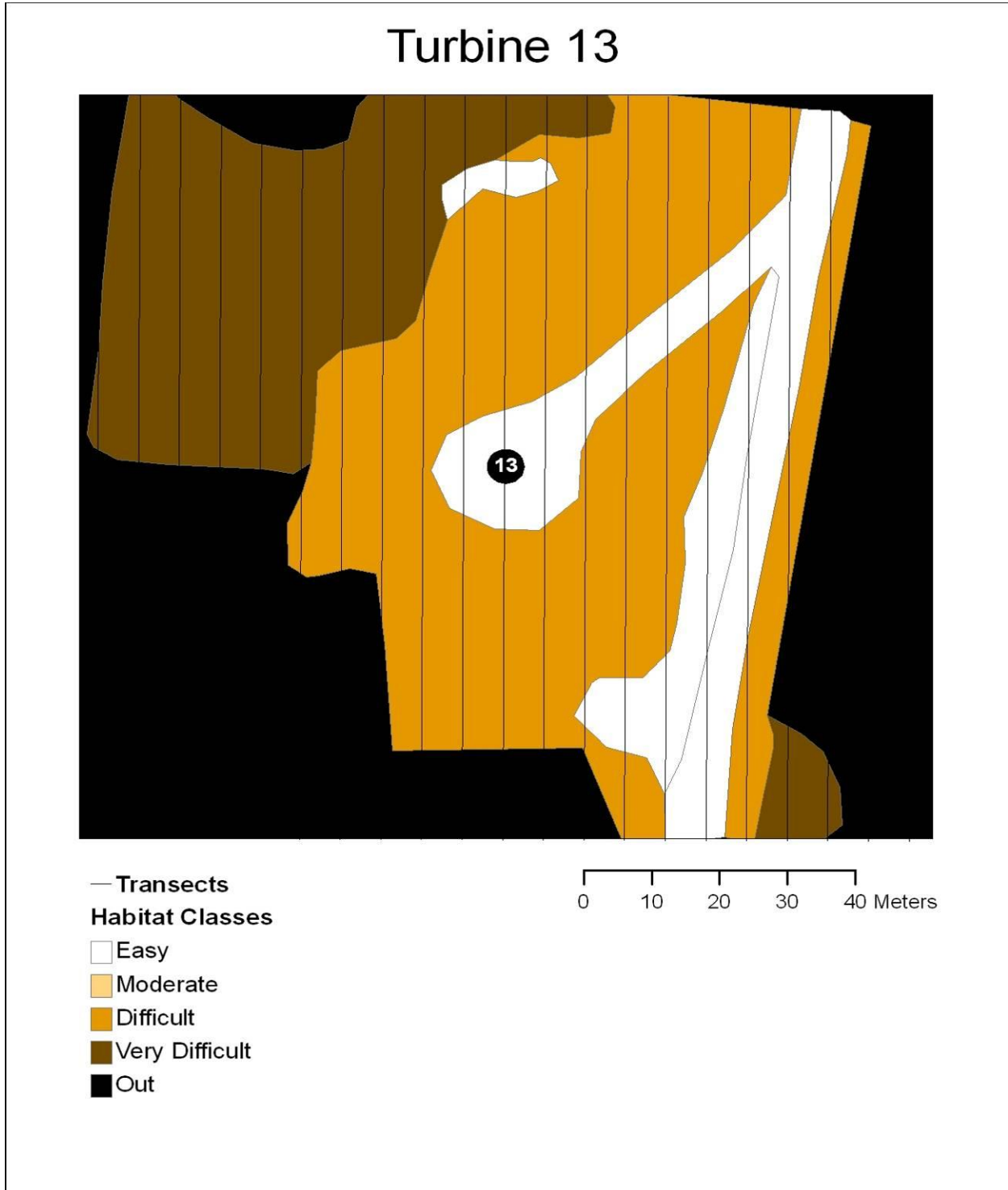
Figure 2. Sample carcass search plot at a wind turbine depicting the maximum plot size of 126 m east-west and 120 m north-south, 6 m wide transect lines (searched 3 m on each side), unsearchable area (black), and area encompassed by easy (white), moderate (light tan), difficult (dark tan), and very difficult (brown) visibility habitat.
