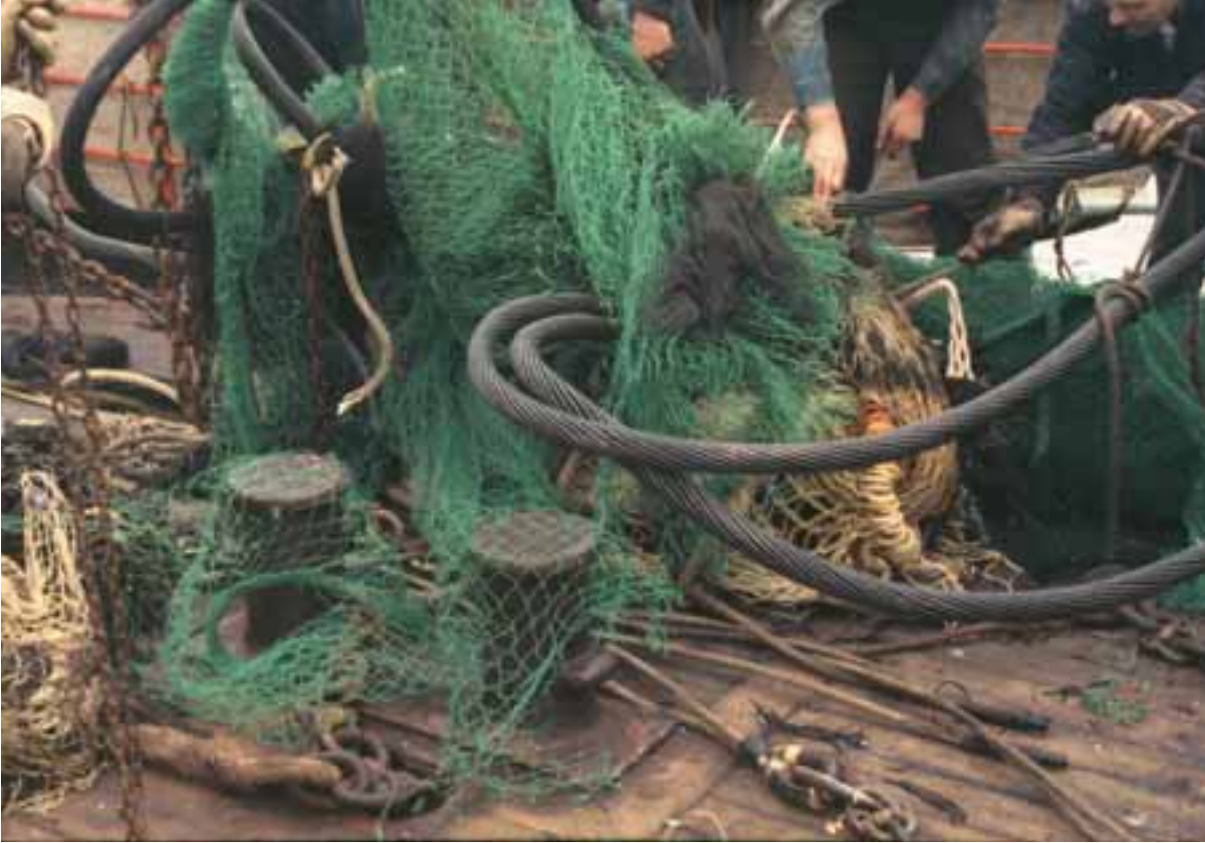
Figure 3.5: Fishing Gear Entangled with an Unprotected Cable System
