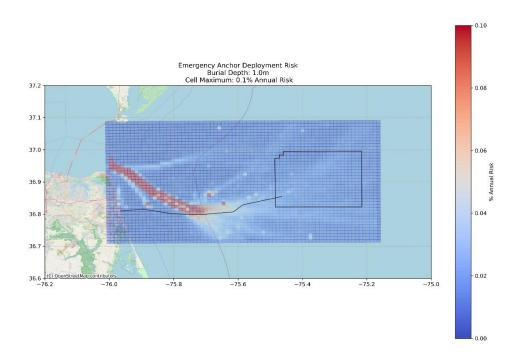
Figure W-52. Area Based Emergency Anchoring Risk Chart, 3.3-ft (1.0-m) Burial Depth
