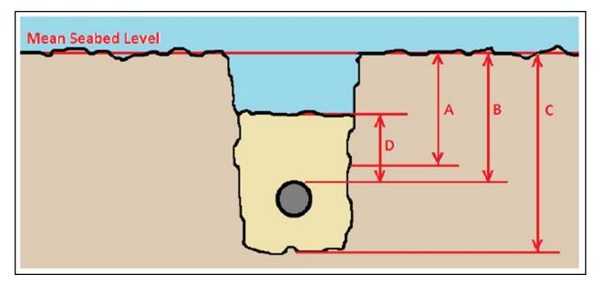
Figure W-10. Trench Definitions (Carbon Trust 2015)
