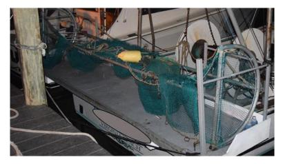
Figure W-20. Beam Trawl, 16 Feet in Width, Secured to the Stern of a Fishing Vessel in Rudee Inlet (Photo Credit: R. Larsen Sea Risk Solutions, LLC)
