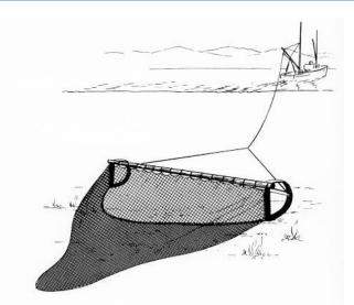
Figure W-19. Schematic of a Beam Trawl (Credit: FAO 2001)
