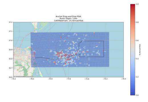
Figure W-57. Area Based Drag & Drop Anchoring Risk Chart, 3.3-ft (1.0-m) Burial Depth
