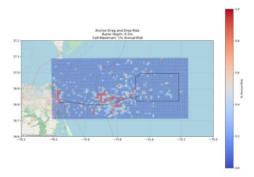
Figure W-56. Area Based Drag & Drop Anchoring Risk Chart, 1.6-ft (0.5-m) Burial Depth
