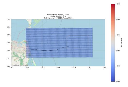
Figure W-59. Area Based Drag & Drop Anchoring Risk Chart, 6.6-ft (2.0-m) Burial Depth
