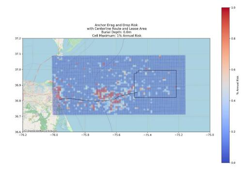
Figure W-55. Area Based Drag & Drop Anchoring Risk Chart, 0-m Burial Depth
