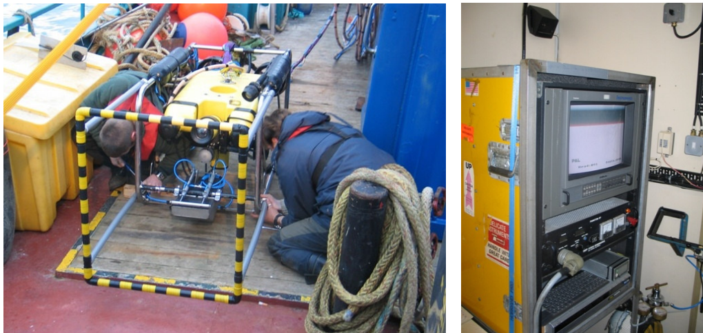
Figure 3. The ROV with the attached PVC device (left) and the ROV control unit on board (right).
