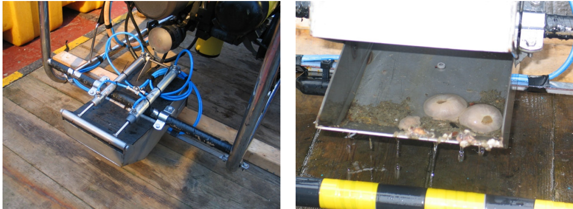
Figure 5. The grab sampler mounted on the ROV (left) and the fouling grabbed from the surface of WTG-07 (right).
