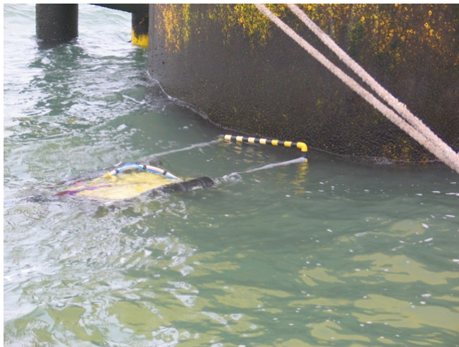
Figure 4. The ROV approaching the WTG-07. At his moment the PVC elongates were still at full length, but needed to be shortened in order to obtain a proper view of the fouling.
