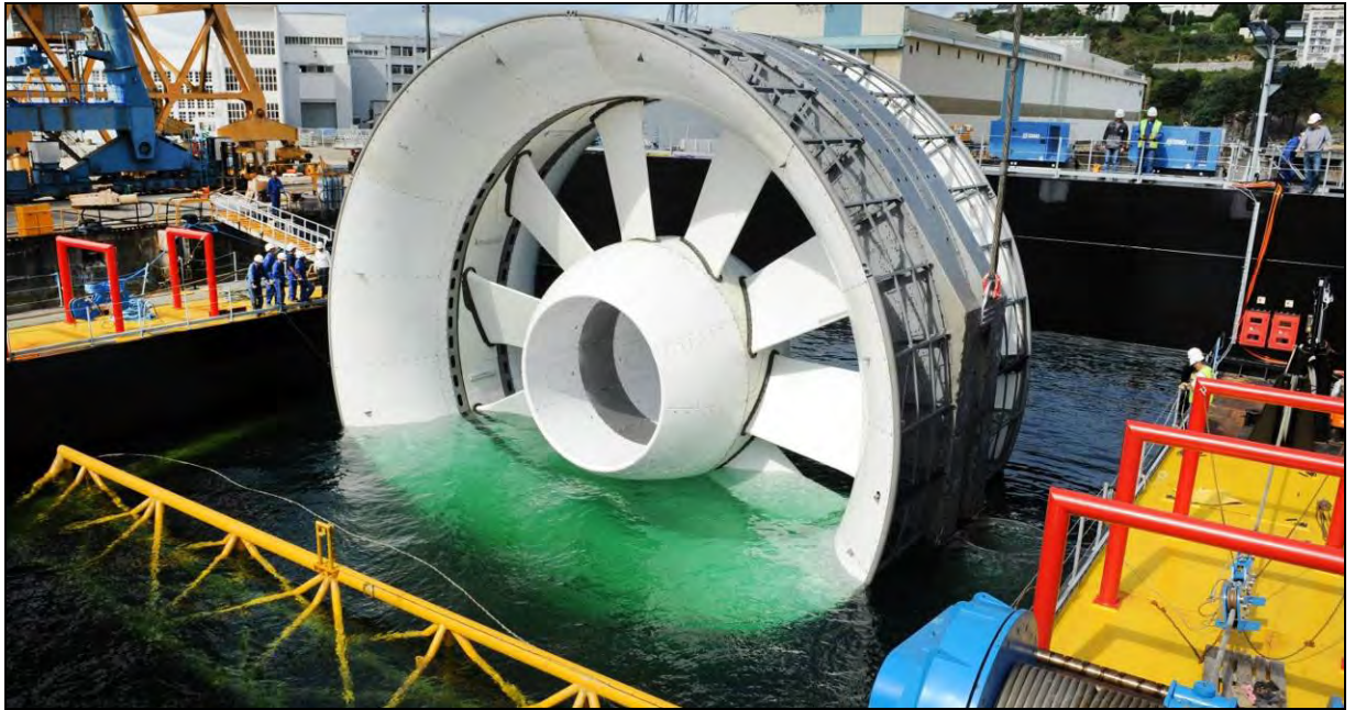
Figure 4.3 - 16m OCT being loaded onto custom-built barge
