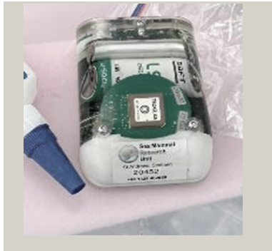
Figure 3. SMRU GPS/GSM (Phone) Tag.
