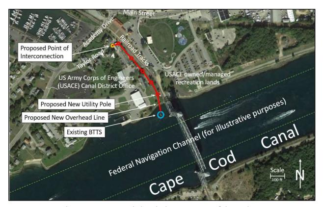
Figure A-6. Proposed Electrical Components of the Project
