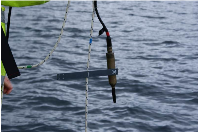
Figure 2-4: Boat-deployed hydrophones (RESON 4032) ready for deployment.
