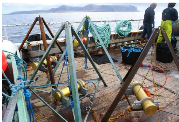
Figure 2-1a): Assembled frames housing DAQ pod and hydrophone on board, with anchor and weight ready for deployment.
