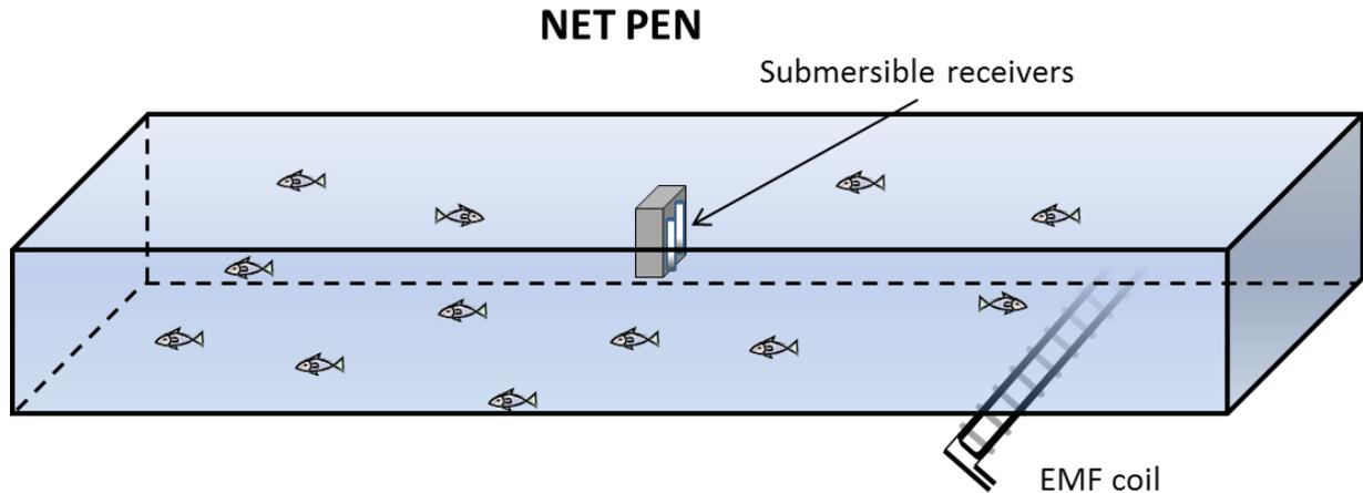
**Fig. 1. The 22  $\times$  7  $\times$  1.5 m net pen was suspended in a 60 $\times$ 10 m pond of similar depth.** Only two of four receivers are shown; the remaining two are not visible on the opposite side of the sound barrier. The EMF coil was connected to the onshore EMF generator system.
