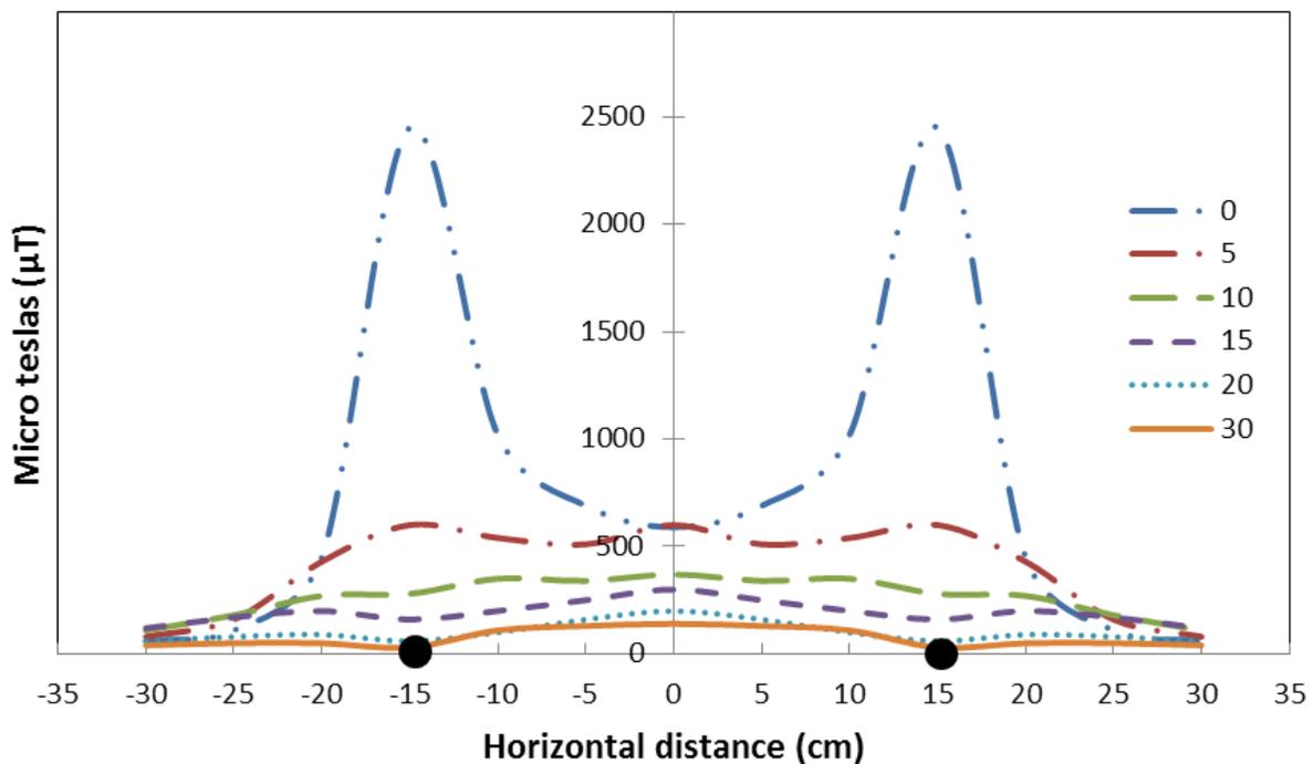
**Fig. 3. Electromagnetic field strength emitted from an experimental cable as measured to either side and above the cable loop.** Along the x-axis, 0 represents the midpoint between the loops of cable, with the cable located at the +15 and -15 locations as indicated by the black dots (i.e., a 30 cm spread). The five lines represent EMF measurements taken at five distances above the horizontal plane of the cable (0 to 30 cm).
