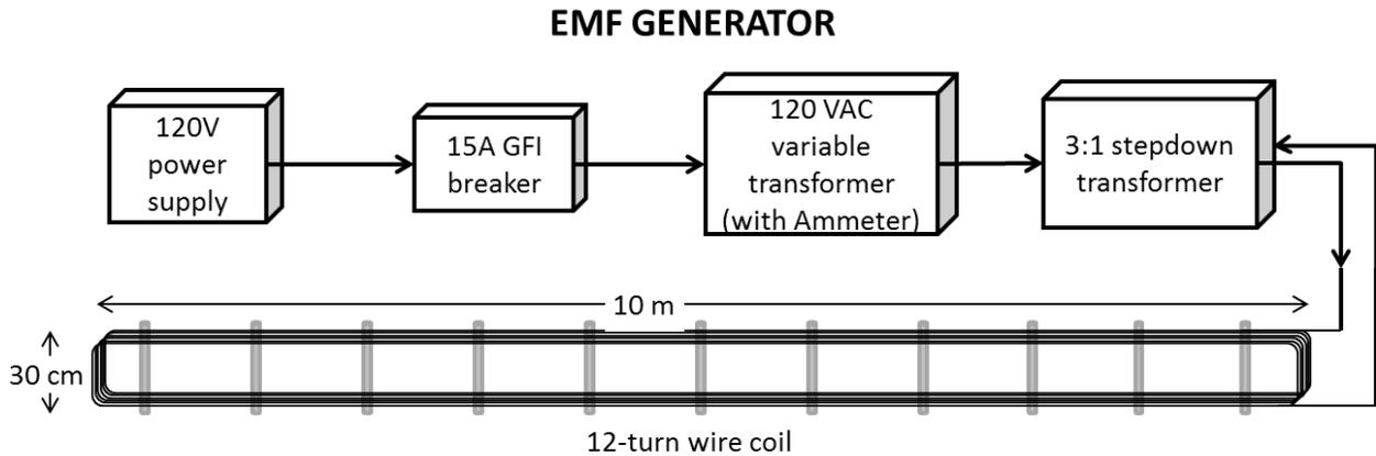
**Fig. 2. Electromagnetic field generator system.** Only the coil was located underwater.
